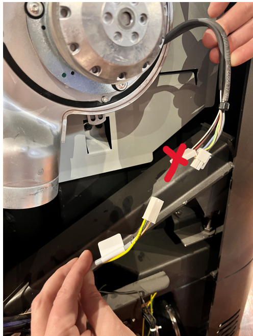
Fig. 5: Connecting the cables
