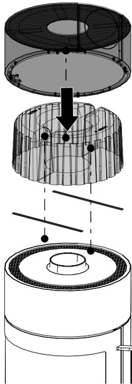
Fig. 1: Installing the HSM bricks
